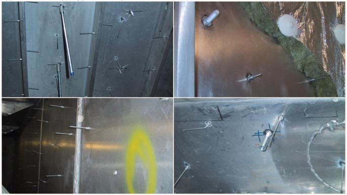
Easy and safe welding of insulation pins using drawn arc welding according to EN ISO 14555
